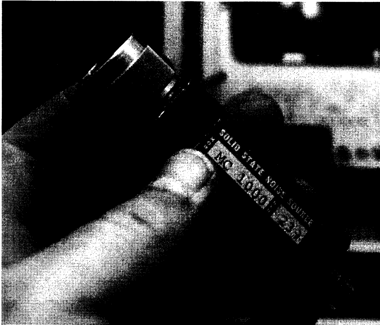
Figure D-2. A typical noise diode solid state noise source. A +28-volt potential applied to the BNC connector on the right produces +24-dB excess noise ratio from the type N connector on the left.
